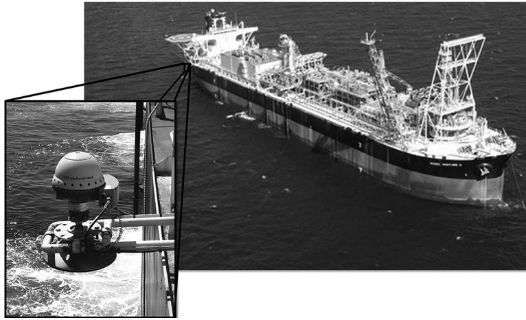
Fig. 1 Example of a vessel with wave-probe on the hull. Adapted from Ref. [1].
